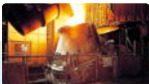
Hikari Steelmaking plant: AOD furnace
