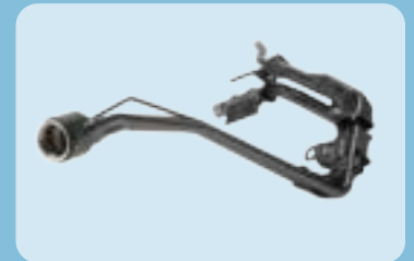
Fuel inlet pipe
