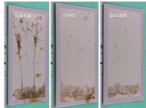
Fig. 10 Appearance after cyclic corrosion cycle test (JASO, 30 cycles), evaluation surface #600
