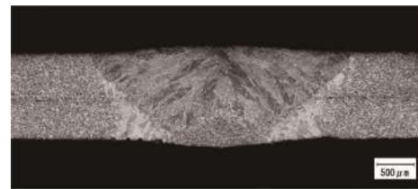
Fig. 9 Optical microscope structure of TIG welding material
